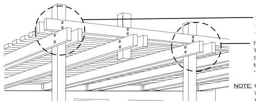
TWO 1/2" DIA. THRU-BOLTS (W/ WASHERS), PER CONNECTION AS SHOWN
